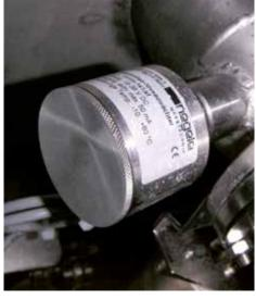
Point level detection in vessels and overfill protection
