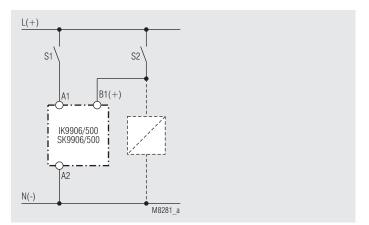
Control with parallel connected load
