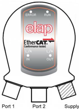
Connectors and LEDs position
