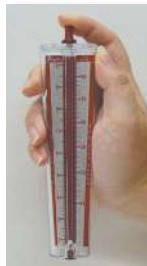
For high scale reading, finger covers hole
