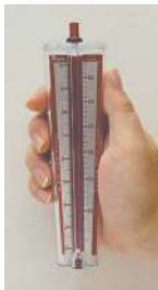
Hold this way for low scale reading
