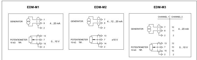
**NOTE:** pin 8 (and 11 for EDM-M3 version) must be connected to pin 15 (0V), when the potentiometer is used as reference signal. This is recommended also when the generator has a pure differential output (not connected to ground).
