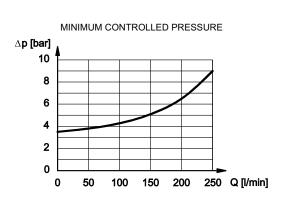
**NOTE**: The maximum flow deliverable to P1 port is 120 l/min (for P2D and P4D modular subplates). The maximum flow through the pressure relief valve (additional 3/4" BSP P port) is 250 l/min.
