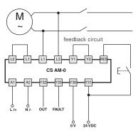
$\bigsqcup$  |  $\bigtriangleup$  | In case of star/delta starting, connect the module to the ends of a single winding For dc motors connect + with L1 and - with L3.
