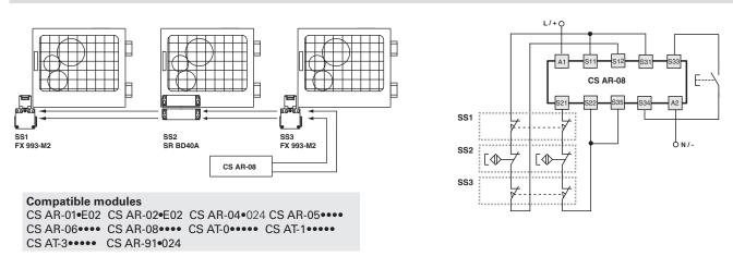
Monitoring of several guards through switches and magnetic sensors. System in category 3. For the calculation of the diagnostic coverage, see ISOTR24119.
