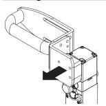
**9750** N The strong interlocking system guarantees a maximum actuator holding force of  $F_{1max} = 9750$  N. This is one of the highest values currently available on the market today, making this device suitable for heavy-duty applications.
