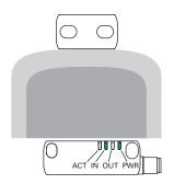
Operating voltage is applied to the sensor, (LED PWR on, green), the inputs are enabled (LED IN on, green), the outputs are deactivated (LED OUT off). The actuator is outside of the actuation zone (LED ACT off).
