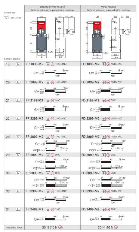
Legend: With positive opening according to EN 60947-5-1, 1 interlock with lock monitoring acc. to EN ISO 14119
