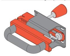
Optional lever for emergency opening from the inside: it ensures that operating personnel can exit the area should they accidentally become trapped within the dangerous area. It can be combined only with switches without lock (e.g. FD •93-M2) or switches with escape release button (e.g. FG •••D6D••).
