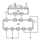
Connections with CS AT-0 •••• / CS AT-1 •••• safety modules
