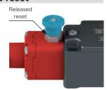
If the tension indicator is in the green area, the electrical safety contacts can be closed by pulling the blue knob. The reset status can be identified guickly by the green ring under the blue knob.
