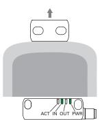
As soon as the actuator exits the limit activation zone, the sensor deactivates the outputs and switches off the OUT and ACT LEDs.
