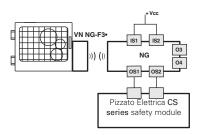
NG series switches can be used as individual devices provided that the safety outputs be evaluated by a Pizzato Elettrica safety module (see table for combinable safety modules).
