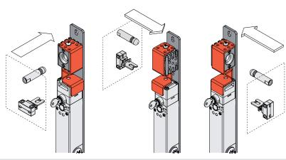
Thanks to its symmetrical design, the lock out device can be installed on hinged and sliding doors, with both right and left closing, while still retaining its centring function and allowing for the attachment of multiple padlocks.
