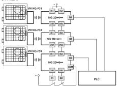
This version, with the IS safety inputs, can be used at the end of a series of NG switches, up to a maximum number of 32 devices, while maintaining the maximum PL e safety level and acc. to EN ISO 13849-1 and SIL 3 safety level acc. to EN 62061.
