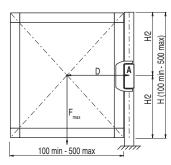
Doors with one safety hinge and one additional hinge (N)=400,000/D (mm)
