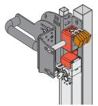
These safety switches alone do not provide sufficient personal protection to the operators or maintenance personnel in situations where they completely enter the danger zone, since unintentional closing of a door after entry could cause the machine to re-start. If the restart release is completely dependent on these switches, a system for preventing this danger must be provided, e.g. a padlockable device for actuator entry locking VF KB2 (page 118) or a safety
