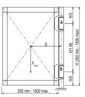
Doors with one safety hinge and two additional hinges <sub>max</sub> (N)=500,000/D (mm)
