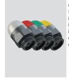
These LED signalling lights are used for signalling that an electric contact has changed its state inside the switch. They can be installed on switches by screwing them on one of the conduit entries not used for electric cables. For details see page 334.
