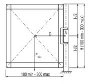
Doors with one safety hinge and one additional hinge F<sub>max</sub>(N)=200,000/D (mm)
