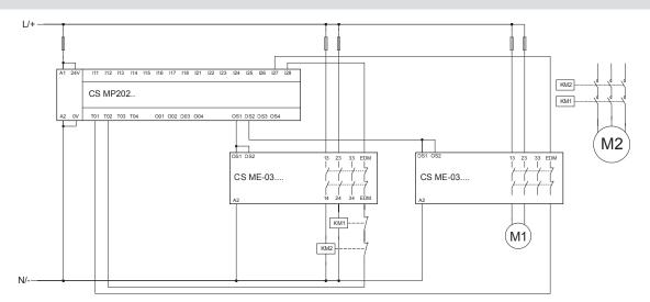
The circuit diagram only shows the connection of the expansion modules; the connection of inputs and other outputs was intentionally omitted. Note: Motor M1 with load according to the utilisation categories of the contacts of the CS ME-03 module.
