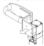
The inside of each switch features a device which holds the actuator in its closed position. Ideal for all those applications where several doors are unlocked simultaneously, but only one is actually opened. The device keeps all the unlocked doors in their position with a retaining force of 30 N, stopping any vibrations or gusts of wind from opening them.
