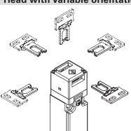
For all switches, the head can be adjusted in 90° steps after removing the two fastening screws. In this way it is possible to actuate the switch from 5 different directions.
