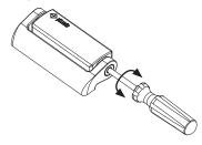
The switching point of the switches can be set with a Phillips head screwdriver.
