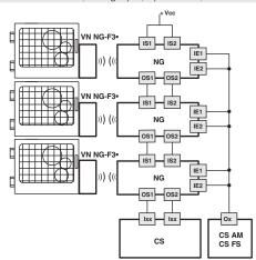
Monitoring function: actuator locked 2 channels / Category 4 / up to SIL 3 / PL e
