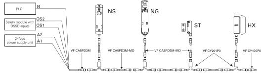
• Attention! For proper operation of the devices connected in series via cables or Y connectors, it is necessary to pay particular attention to the voltage drop that occurs in the circuit. Pay particular attention to the currents and cross-sections/lengths of the used cables to ensure that the supply voltage of the components at the end of the series connection remains within the specified limit values during effective operation.
