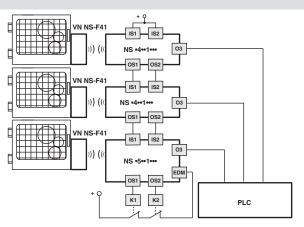
This version, with the IS safety inputs, can be used at the end of a series of NS switches, up to a maximum number of 32 devices, while maintaining the maximum PL e safety level and acc. to EN ISO 13849-1 and SIL 3 safety level acc. to EN 62061.
