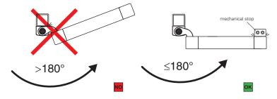
The actuator must not strike directly against the magnetic sensor.
