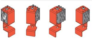
With a single operation, the lock out device enables the closure of both the centring hole and the slot for the actuator present in the switch, thus making the mechanical closure of the door and the electrical commutation of the switch contacts impossible.
