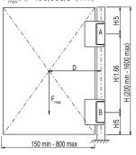
Doors with one safety hinge and two additional hinges
