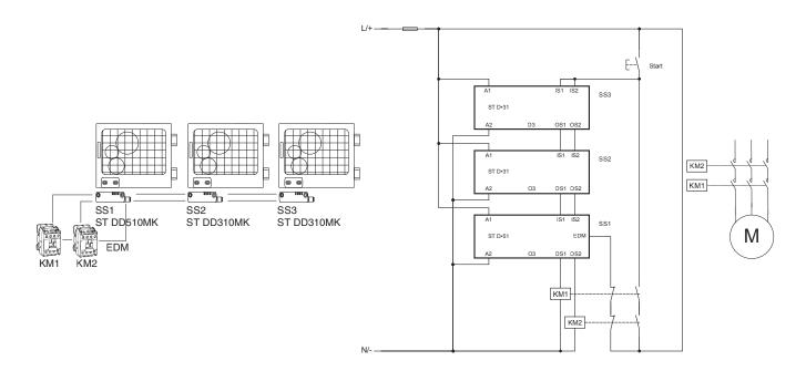
Direct monitoring of the status of the contactors via the EDM input of the last sensor in the series connection
