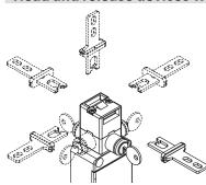
The head can be quickly turned to each of the four sides of the switch by unfastening the two fastening screws.
