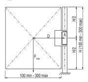
Doors with one safety hinge and one additional hinge  $F_{max}(N)=100,000/D \text{ (mm)}$
