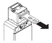
The robust interlocking system guarantees a maximum actuator holding force of  $F_{\rm 1max} = 1100~{\rm N}.$
