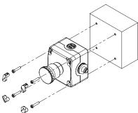
The wall fixing screws and the ones for closing the housing cover can be sealed with 4 caps (supplied with the housing). The caps not only give the housing a more pleasant look, but they also prevent the accumulation of dirt inside the recesses of the screws besides making tampering more difficult.
