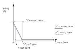
**Contact block with snap action:** 2, 3, 17 The pressure on the contacts decreases as the switching point is approached
