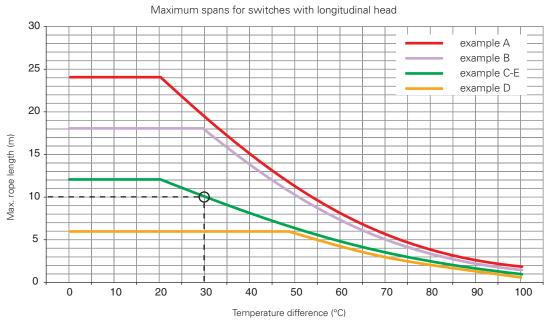
The max. recommended spans are indicated in the diagram as a function of the temperature fluctuations (temperature differences) to which the switch may be exposed at the point of use. For instance, with installation of type C and a temperature difference of 30°C, the max. recommended rope length is 10 metres.
