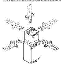
For all switches, the head can be adjusted in 90° steps after removing the two fastening screws. In this way it is possible to actuate the switch from 5 different directions
