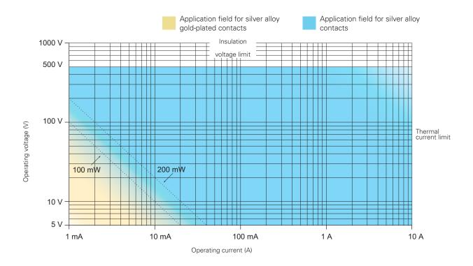
**100 mW** Suggested limit for general applications with snap action contact blocks with silver alloy contacts.
