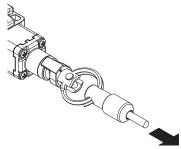
These switches can be supplied with reduced hardness internal springs on request. The force required to actuate the switch can thereby be reduced without changing the actuating path of the electrical contacts. This is particularly advantageous for smaller spans, but must, however, always make use of rope pulleys.
