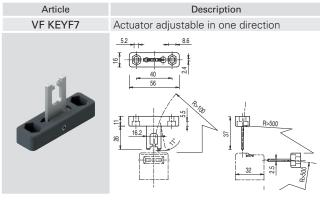
Actuator adjustable in one direction for guards with reduced dimensions.
