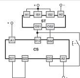
Connection with safety module CS MP ••••0
