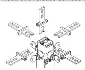
The head can be quickly turned to each of the four sides of the switch by unfastening the two fastening screws.
