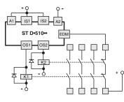
The ST D•51••• version, in addition to maintaining the operating and safety characteristics of the ST series, allows control of forcibly guided NC contacts of contactors or relays controlled by the safety outputs of the sensor itself. As an alternative to the relays or contactors you can use Pizzato Elettrica expansion modules CS ME-03. See page 263.
