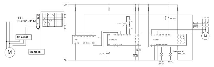
Guard monitoring and interlock by means of interlocking device with RFID technology in category 4, PL e and SIL3. Release command enabled by the safety module for standstill monitoring.
