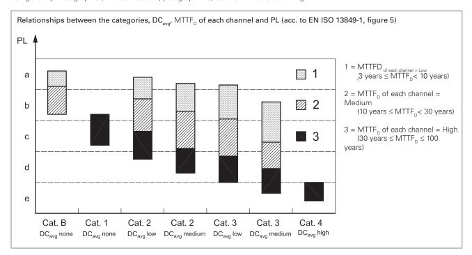
This figure is very useful, as it can be read from multiple points of view. For a given  $PL_r$ , it shows all possible solutions with which this PL can be achieved, i.e., the possible circuit structures that provide the same PL.
