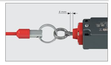
For switches with head 74: Tighten the rope connected to the switch until the thimble will be at about 4 mm from the head.
