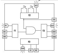
Function f0 is a basic function and includes the monitoring of the power supply as well as internal, cyclical tests.
