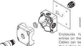
Enclosures have 2 conduit entries on the lower surface. Cables can be connected via this surface, hiding them from view.
