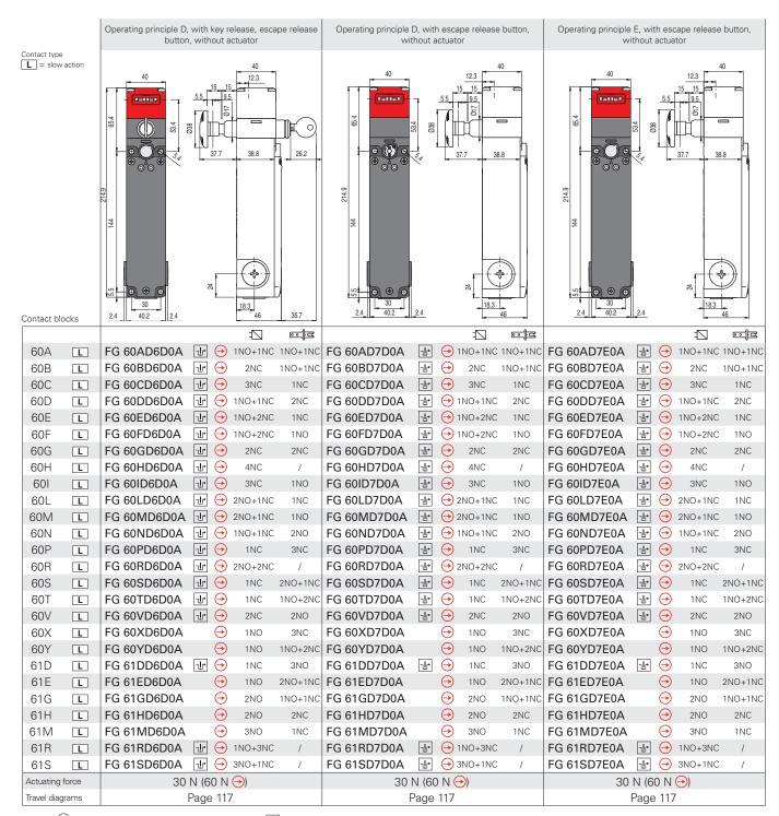
Legend: With positive opening according to EN 60947-5-1, 1 interlock with lock monitoring acc. to EN ISO 14119
