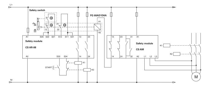
NOTE: The NC contacts of K1 and K2 are mechanically guided (EN 60947-4-1, Annex F)
