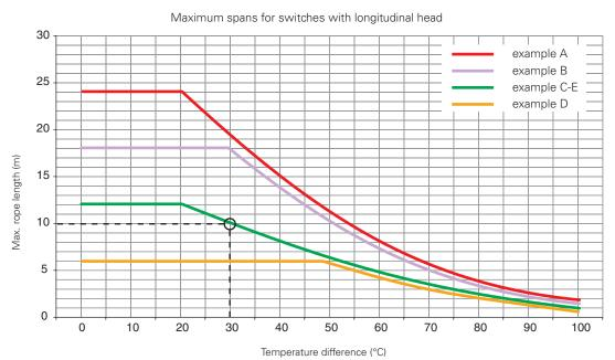
max. recommended spans are indicated in the diagram as a function of the temperature fluctuations (temperature differences) to which the switch may be exposed at the point of use. For instance, with installation of type C and a temperature difference of 30°C, the max. recommended rope length is 10 metres.
