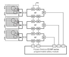
Possibility of series connection of multiple sensors for simplifying the wiring of the safety system, whereby only the outputs of the last sensor are evaluated by a Pizzato Elettrica safety module of the CS MP series. Both the safety-relevant evaluation and the evaluation of the signalling outputs are performed by the CS MP series.
