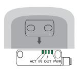
If the actuator is moved inside the safe activation zone (dark grey area), the ACT LED on the sensor illuminates (green) and it activates the outputs (LED OUT on, green).
