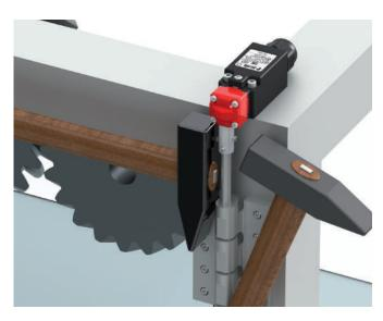
Pin the switch (pin is provided).
