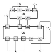
Connections with CS AR-05 •••• / CS AR-06 ••• safety modules
