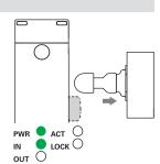
When the actuator leaves the actuation limit area, the device turns off the ACT LED and the O3 signalling output.
