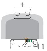
When the actuator leaves the safe zone, the sensor keeps the safety outputs enabled. Entry into the limit activation zone (light grey area) is, however, indicated by the ACT LED (orange/green, flashing).
