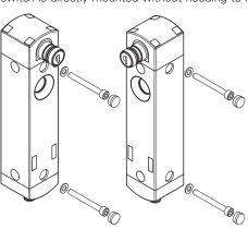
contains the hole for inserting the actuator pin. The fixing holes can be sealed with the protection caps provided for this purpose. Dirt deposits and tampering attempts are thereby prevented.
