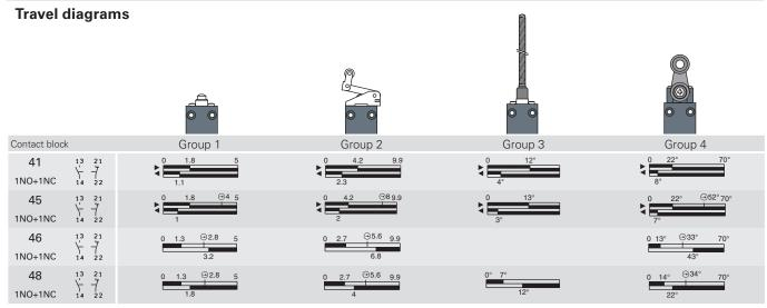
Legend Closed contact | ☐ Open contact | ③ Positive opening travel acc. to EN 60947-5-1 | ▶ Switch pressed / ◀ Switch released
