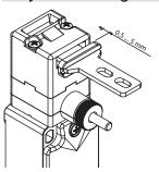
The actuation head of this switch features a wide range of travel. In this way the guard can oscillate along the direction of insertion (4.5 mm) without causing unwanted machine shutdowns. This wide range of travel is available in all actuators in order to ensure maximum device reliability.
