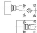
The switch is provided with a wide centring inlet for the actuator pin. This solution makes it easier to align the actuator and the opening hole on the head during installation. Moreover, this solution drastically reduces the probability of a collision between the switch and the actuator, making it possible to install the device even on inaccurately closing doors.
