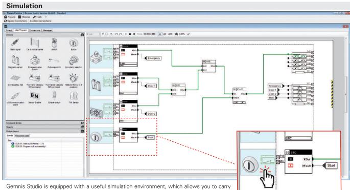
Gemnis Studio is equipped with a useful simulation environment, which allows you to carry out tests on your application program under development and check its correct operation before you install it in a module. To run an application program simulation during the develop-
