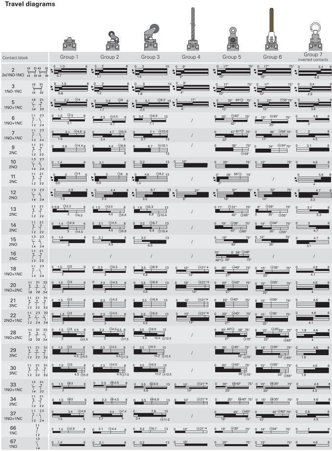
(\*) Positive opening of NC contacts (11-12 / 21-22 / 31-32) with 22 actuator with rigid rod only. Do not operate the 22 actuator with rigid rod at an angle of more than 27°
