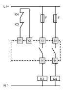
If necessary the number and the load capacity of output contacts can be increased by using expansion modules or contactors with forcibly guided contacts. For control of the external contactors, a NC contact of each relay is connected to the safety module feedback circuit between the start button terminals.
