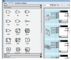
The function blocks represent all the logic functions required to process the data flow between sensors and outputs.
