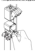
As soon as the lock out device has been actuated and locked, the slot in the switch for the actuator is no longer accessible.
