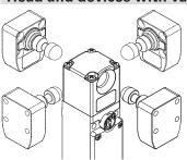
The system can be variably configured by loosening the 4 screws on the head.
