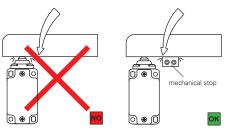
The guard must not use the switch head as a mechanical stop.
