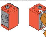
With a single operation, the lock out device can close the centering hole, making it impossible to mechanically close the door.
