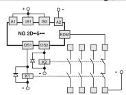
The NG 2D••5•••version, in addition to maintaining the operating and safety characteristics of the NG series, allows control of **forcibly guided NC contacts of contactors or relays** controlled by the safety outputs of the switch itself. As an alternative to the relays or contactors you can use Pizzato Elettrica expansion modules CS ME-03. See page 267. This check is carried out via the EDM input (External Device Monitoring as defined in EN 61496-1) of the switch.
