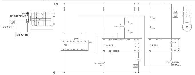
Guard monitoring and interlock by means of interlocking device with RFID technology in category 4, PL e and SIL3. Release command enabled by the safety timer.
