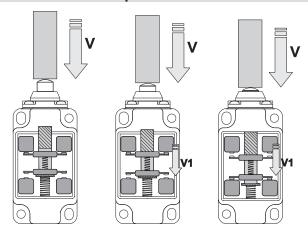
Contact block with snap action: component where the speed of the contact movement (V1) doesn't depend on the speed of the switch actuation (V). Upon reaching a predetermined point in the actuation travel, the contact carrier triggers and switches the contacts
