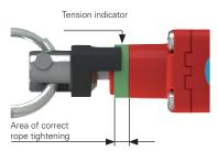
All switches are provided with a green ring that shows the area of the correct tightening of the rope. The installer has only to tighten the rope until the black indicator will be in the middle of the green area. With this setting, the switch can be reset by pulling the blue knob to close the electrical safety
