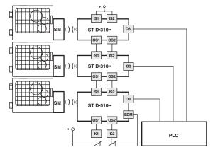
This version, with the IS safety inputs, can be used at the end of a series of ST sensors, up to a maximum number of 32 devices, while maintaining the maximum PL e safety level according to EN ISO 13849-1.
