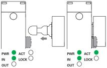
The switch is supplied with power (PWR LED on, green), the IS1 and IS2 inputs are enabled (IN LED on, green), the OS1 and OS2 safety outputs are disabled (OUT LED off). The actuator is outside of the actuation zone (LED ACT off).
