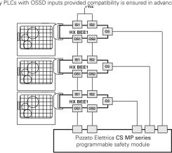
Possibility of series connection of multiple hinges for simplifying the wiring of the safety system, whereby only the outputs of the last hinge are evaluated by a Pizzato Elettrica safety module of the CS MP series. Both the safety-relevant evaluation and the evaluation of the signalling outputs are performed by the CS MP series.
