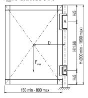
Doors with one safety hinge and two additional hinges F<sub>max</sub> (N)=250,000/D (mm)
