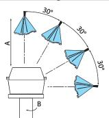
ISO 20653 envisages a particularly strenuous test. This test simulates the conditions of pressure washing in industrial environments with water jets having pressure between 80 and 100 bar, flow rate between 14 and 16 l/min. and a temperature of 80°C.
