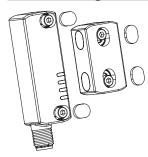
Each sensor and actuator of the ST series is supplied complete with snapon protection caps to be applied on the holes of the fixing screws. Not only do the caps prevent dirt from accumulating and simplify cleaning, they also block access to the fastening screws of the actuator. As a result, standard screws can be used instead of tamperproof screws.
