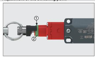
For switches with head 79 and 80: Tighten the rope connected to the switch, until the end of the indicator (1) reaches about the middle of the green ring (2).
