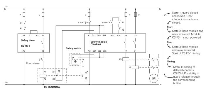
The diagram illustrates the operating principle of a typical circuit for monitoring a door-lock system with interlock in the de-energised state and manual release of the individual doors.
