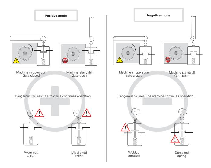
With positive mode, preventive maintenance can be performed, thereby avoiding the dangerous failures described above. With negative mode, on the other hand, failures can occur within the switch and are therefore difficult to detect.
