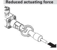
These switches can be supplied with reduced hardness internal springs on request. The force required to actuate the switch can thereby be reduced without changing the actuating path of the electrical contacts. This is particularly advantageous for smaller spans, but must, however, always make use of rope pulleys.
