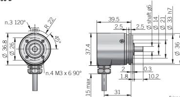
recommended mating shaft tolerance H7 dimensions in mm
