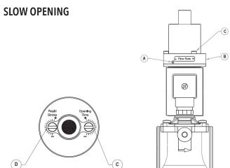
Flow rate adjustment. Loosen screw A and rotate cylinder B to the desired position. Tighten screw A to fix the position.
