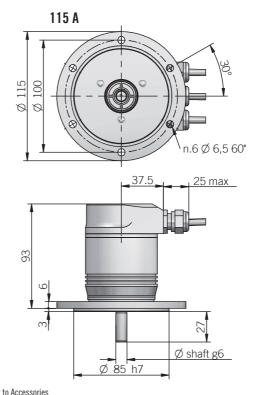
recommended mating shaft tolerance H7 dimensions in mm
